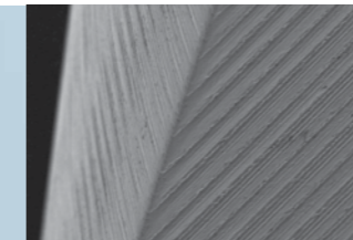
Circumferential cutting edge, slightly rounded 3 µm
